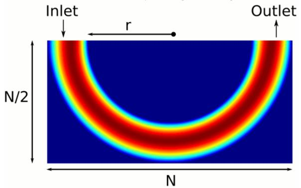
The fluid is confined in a channel shaped like a half-circle. Pressure boundary conditions are used with an appropriate difference
